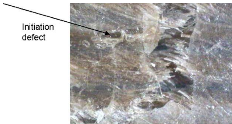
Figure 2 Propagation of impact damage in flax-epoxy (0.9 mm thread) laminate from a sub-surface defect.
