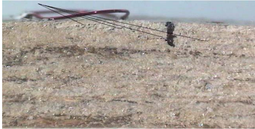
Figure 3 Sub-surface defects in a flax-epoxy laminate.
